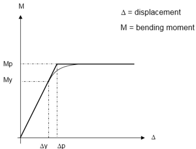
Figure 1 – Material Behavior for Plastic Hinge Analysis
