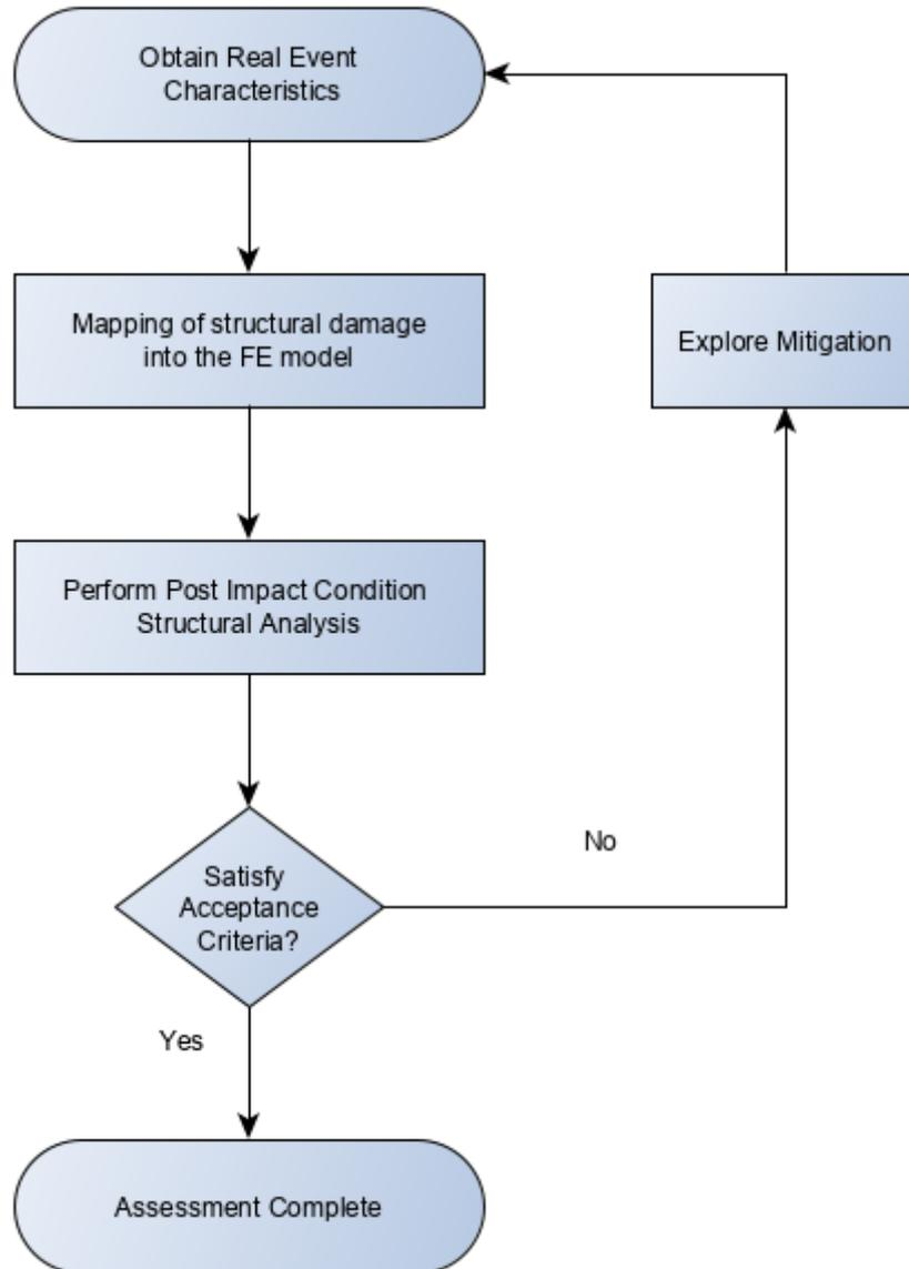
Figure 3 – Post Impact Condition Assessment Process
